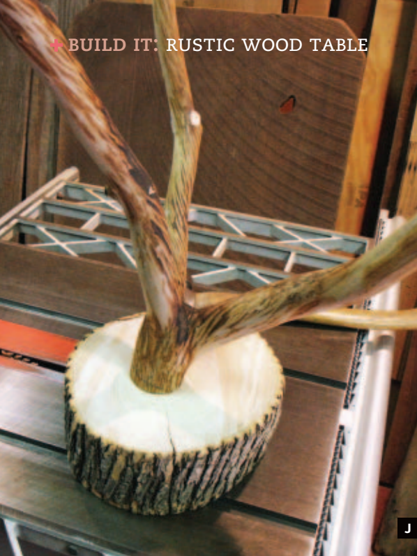
Fig. J: The base and underside of the top are attached together with the dowel screw. Make sure to tighten securely.
