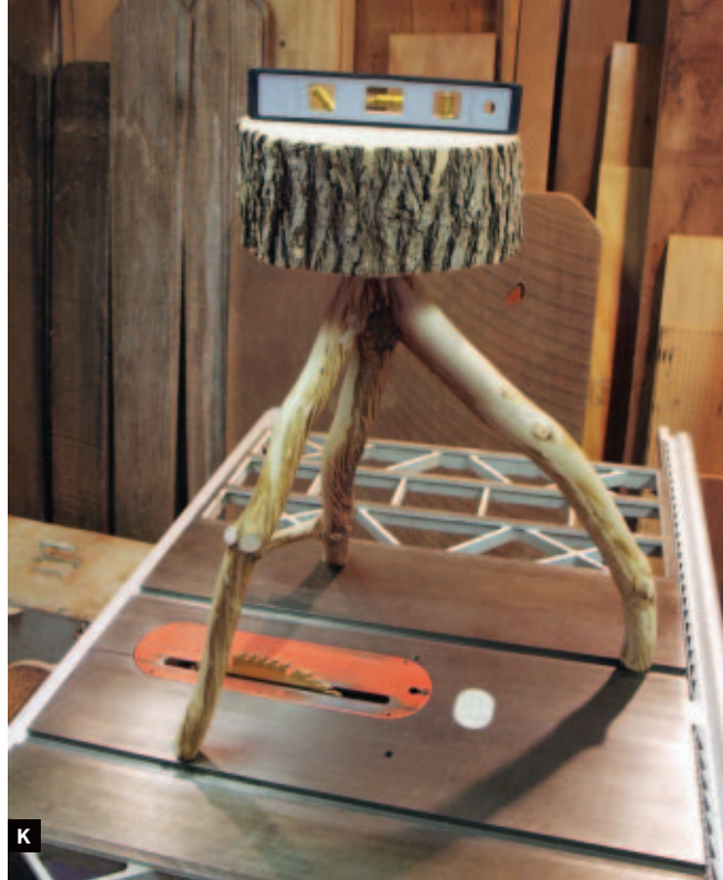
Fig. K: Use a level to make sure your creation doesn't tilt to one side. Don't assume that your floor is true.
