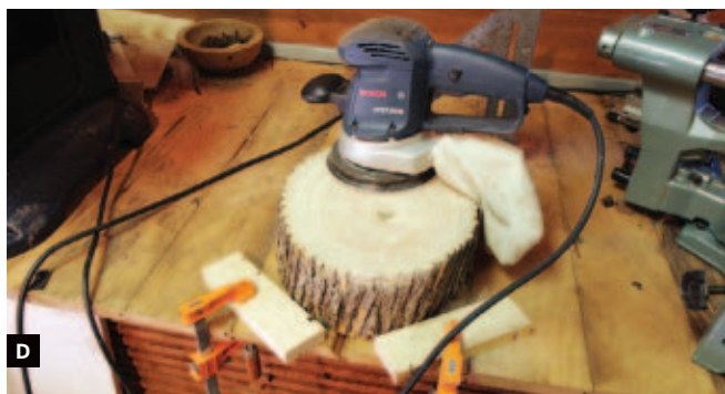
Fig. C: Evening out the top with a belt sander. Note the wood blocks used to secure it. Fig. D: Fine sanding with an orbital sander makes the top silky smooth.
