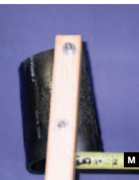
Fig. I: Each footplate sits on the peg so that the shin support is on the outside the shin. Fig. J: Pre-drill and attach the footplate with wood screws. Fig. K: Cut out a 3"-wide vertical section of each ABS piece. Fig. L: Fit the ABS
