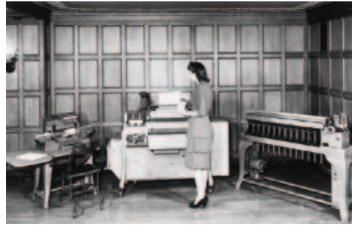
FAR LEFT: The Jacquard loom, which used punch cards to store weaving patterns, revolutionized the weaving industry. LEFT: Paper punch cards for computers were modeled after the Jacquard loom's wooden cards. ABOVE: This punch-card reader from the mid-20th century reads data on computer cards, working on the same principle as the Jacquard loom.
